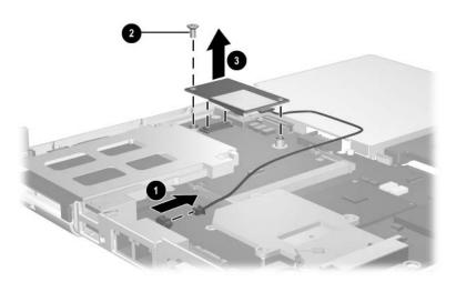
Removing the Modem Board
